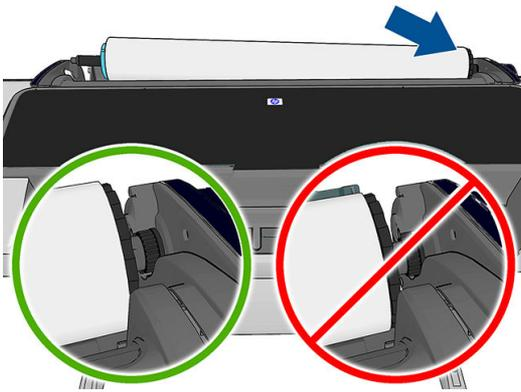
5. Rest the blue end of the spindle on the right side roll holder.
