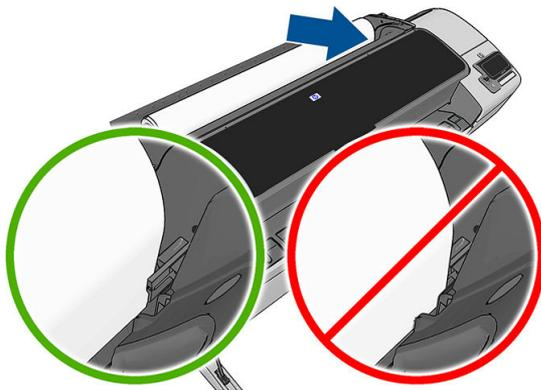
9. Roll the paper into the printer until you feel resistance and the paper flexes slightly. When the printer detects the paper, it feeds it in automatically.
