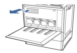
NOTE: Maintain the position of the TCU as you pull it out from the printer. This will ensure that you do not spill any waste toner in the printer. Place the unit into the clear plastic bag the new TCU was packaged in.
