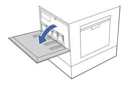
2. Lift the TCU slightly and then pull it out of the printer.
