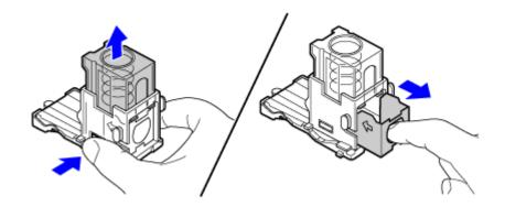
When staples remain, the staple cartridge cannot be removed.
