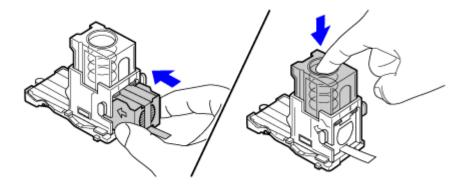
Do not remove the seal from the cartridge before inserting the cartridge into the case.
