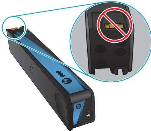
3. If you see any scratches, or other damage on the metal connector, replace the ink cartridge.
