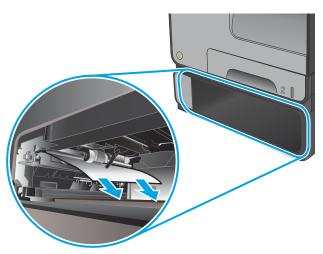
3. If the jam cannot be cleared at the tray, try clearing the jam from the lower left door.
