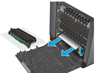
3. If the paper is not visible or accessible, remove the ink collection unit by pulling it out with both hands. Set the unit aside, upright, on a piece of paper to prevent ink spills.
