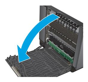
2. Gently remove any visible paper from the rollers and delivery area.
