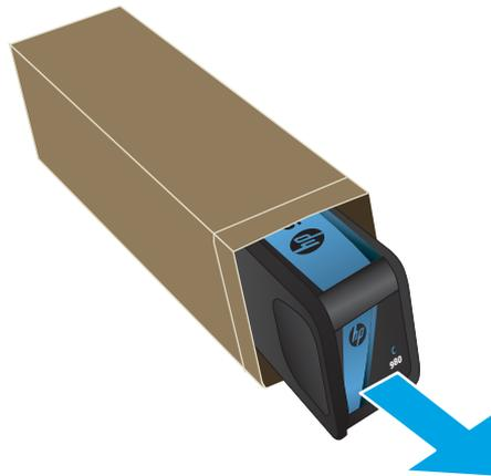
5. Do not touch the gold-colored metal contacts of the ink cartridge. Fingerprints on the contacts can cause print-quality problems.
