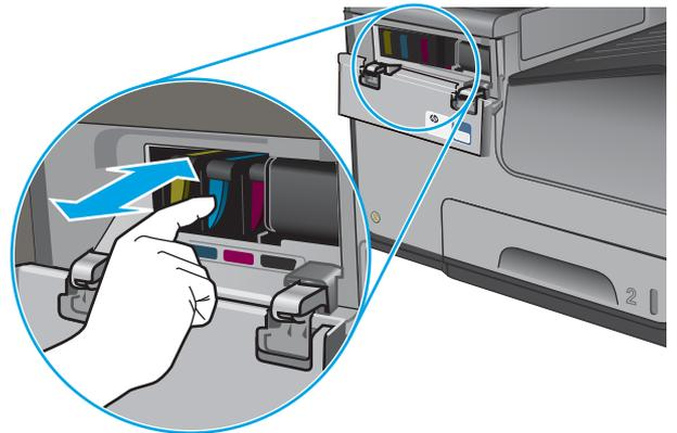
3. Grasp the edge of the old ink cartridge and then pull the cartridge straight out to remove it.
