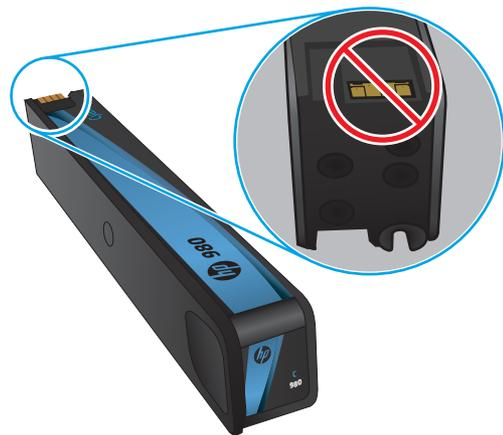
6. Insert the new ink cartridge into the product. Push the cartridge until it clicks into place.
