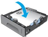
4. Push down on the paper to make sure that the paper stack is below the paper limit tabs on the side of the tray.
