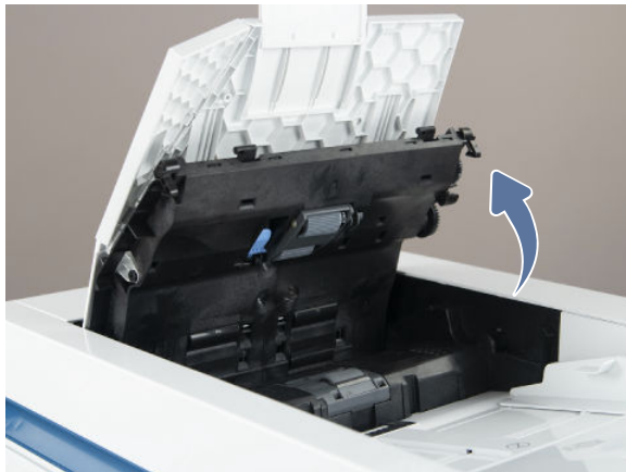
Figure 9-10 Open the document-feeder jam access door
