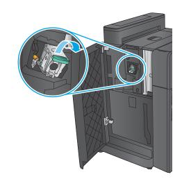
**4.** Lift up the metal handle on the front of the staple cartridge.
