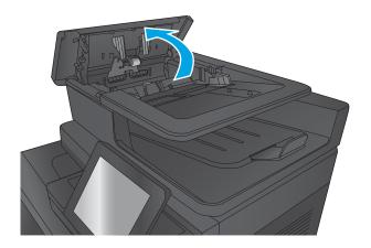
3. Lift the jam-access door, and remove any jammed paper.
