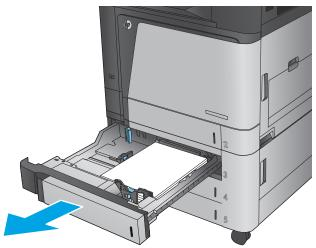
Remove any jammed or damaged sheets of paper.
