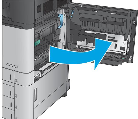
2. Lift the green handle on the transfer-access panel and open the panel.
