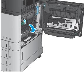
4. Lift the jam-access cover at the bottom of the duplex printing path, and remove any jammed paper.
