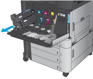
**3.** Remove the new imaging drum from its protective bag.
