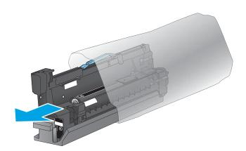
4. Align the imaging drum with its slot, and then insert the imaging drum into the product. The protective cover on the bottom of the drum automatically slides off as the imaging drum is inserted. Recycle this cover with the used imaging drum.
