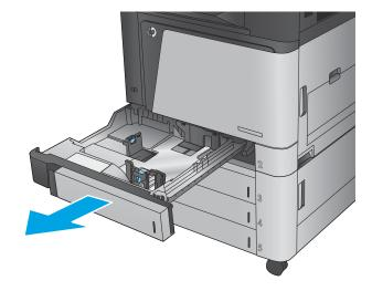
Adjust the paper-length and paper-width guides by squeezing the adjustment latches and sliding the guides to the size of the paper being used.
