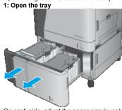
On each side, adjust the paper-size lever to the correct position for the paper you are using.
