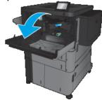
2. Push the button on the lever, and then rotate the toner-cartridge lever to the down position.
