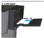
Make sure that the paper fits under the fill line on the paper guides.
