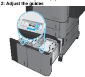
3. Load full reams of paper into each side of the tray. The right side holds 1,500 sheets of paper. The left side holds 2,000 sheets of
