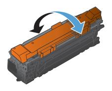
Remove the orange protective cover from the print cartridge.
