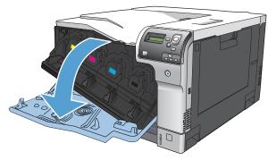
Grasp the handle of the used print cartridge and pull out to remove.
