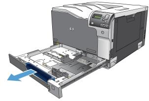
Adjust the paper-length and paper-width guides by squeezing the adjustment latches and sliding the guides to the size of the paper being used.
