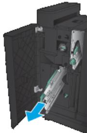
5. Pull the green handle of the stapler unit toward you and rotate it upward. Push the handle in to lock in the open position.
