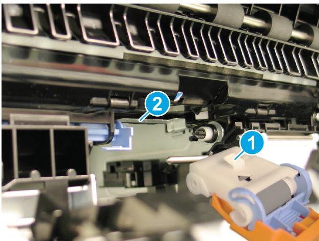
**EN** **NOTE:** The white hook on the top of the roller assembly (callout 1) will hook onto a sheet metal plate (callout 2) when installed correctly.
