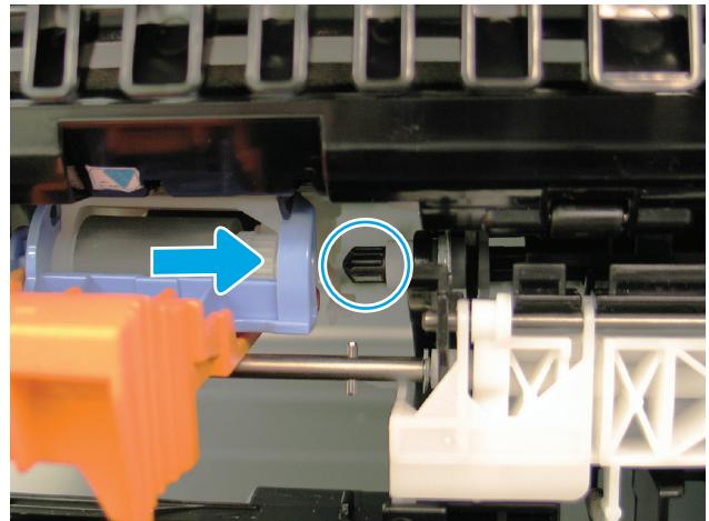
**EN** Align the arrow on the roller assembly with the arrow in the printer, and then slide the rollers into the printer. Slide the rollers to the right onto the black shaft.
