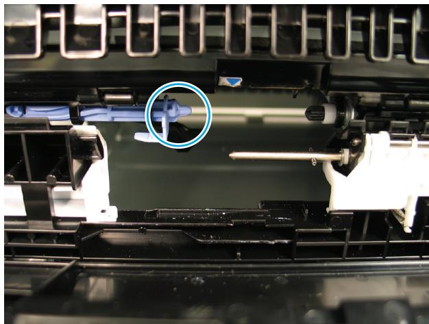
**EN** **NOTE:** If the left post does not stay in the locked position, press the end of the post left until it clicks into place.
