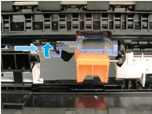
**EN** Locate the lever on the blue shaft on the left, and then release the lever by pressing upward. The blue shaft should spring to the right to click into position to hold the rollers in place. Remove the orange tool by pulling it away from the printer.
