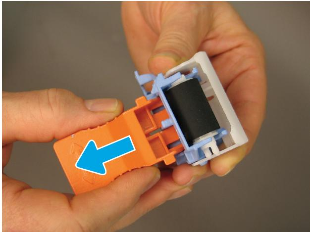
**EN** Remove the orange tool from the roller.
