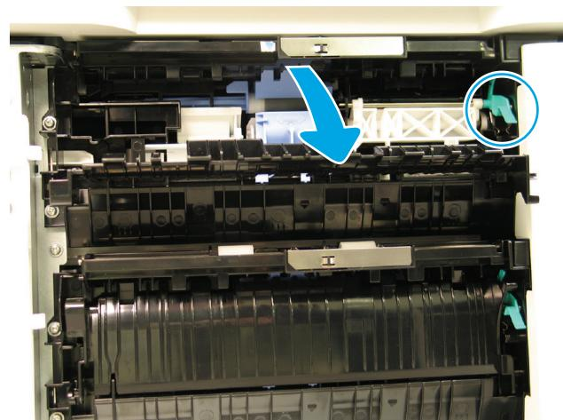
**EN** Open the right door of the paper feeder. Locate the green tab on the feed assembly cover. Release the tab to lower the assembly cover.
