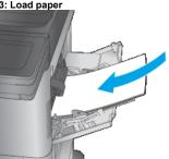
4. Make sure that the paper fits under the fill line on the paper guides.
