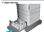
Adjust the paper-width guide to the correct position for the paper.
