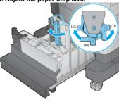
4. Load paper into the tray. Check the paper to verify the guides lightly touch the stack, but do not bend it.
