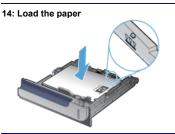
If the tray is not adjusted correctly, an error message might appear during printing or the paper might jam.
