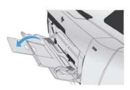
4. Extend the paper guides fully (1) and then load the paper stack into tray 1 (2). Adjust the paper guides to the size of the paper. 4: Open the paper guides
