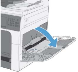
2. Pull out the tray extension to support the paper and set the side guides to the correct width. 10: Location of the tray extension
