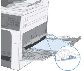
Adjust the side guides so that they lightly touch the paper stack but do not bend it. 13: Load paper
