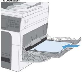
Make sure the stack fits under the tabs on the guides and does not exceed the load-level indicators.
