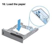
If the tray is not adjusted correctly, an error message might appear during printing or the paper might jam.
