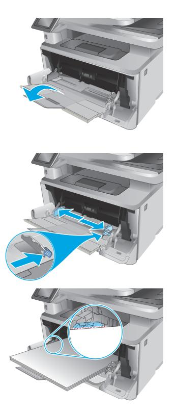
6. Press down on the tab on the right paper guide, and then adjust the paper guides so that they lightly touch the paper stack but do not bend the paper.
