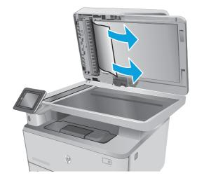
7. Open the scanner lid. If paper is jammed in the scanner lid, gently pull it out, and then close the scanner lid.
