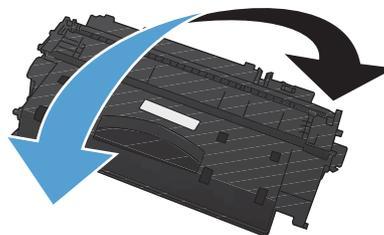
4. Bend the tab on the left side of the cartridge until the tab breaks loose. Pull the tab until all the tape is removed from the cartridge. Place the tab and tape in the toner cartridge box to return for recycling.
