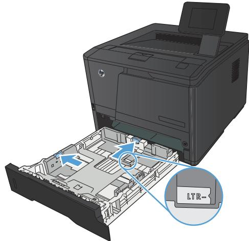
3. To load Legal-size paper, extend the tray by pressing the release button at the back of the tray inward and pulling the back of the tray out.
