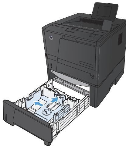
3. To load Legal-size paper, extend the tray by pressing the release button at the back of the tray inward and pulling the back of the tray out.
