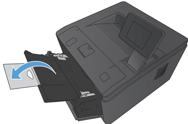
3. Place the paper stack into Tray 1, and slide the paper guides so that they are against the sheets.
