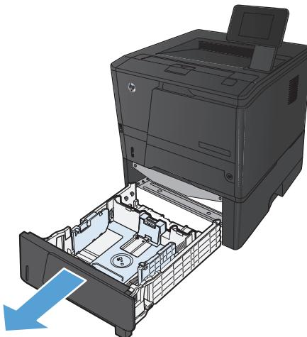
2. Slide open the paper length and width guides by pushing outward on the blue tabs.
