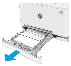
2. Remove any jammed or damaged sheets of paper.
