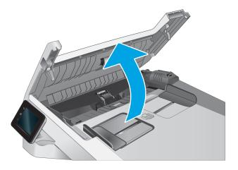
2. Use a moist, lint-free cloth to wipe both pickup rollers and the separation pad to remove dirt.
