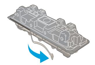
5. Remove the toner cartridge from the opened packaging shell. Save all packaging for recycling the used toner cartridge.
