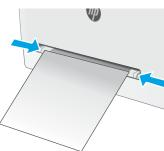
3. Insert the single sheet into the slot and hold it. The printer will pull the sheet partially into the paper path. For information about how to orient the paper, see <a href="Tray 1">Tray 1</a> paper orientation on page 16.
