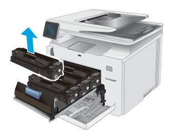
4. Remove the new toner cartridge package from the box, and then pull the release tab on the packaging.
