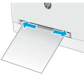
2. Place the top edge of the sheet at the opening, and then adjust the side guides so that they lightly touch the sheet, but do not bend it.
