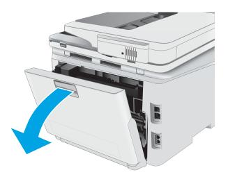
2. Remove any jammed or damaged sheets of paper.
