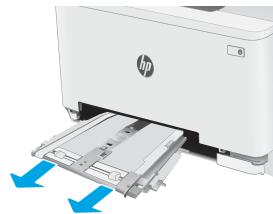
3. Gently pull any jammed paper straight out of the single-sheet priority feed slot.
