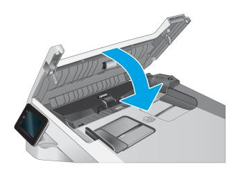
Lift the document feeder input tray to provide better access to the document feeder output bin, and then remove any jammed paper from the output area.
