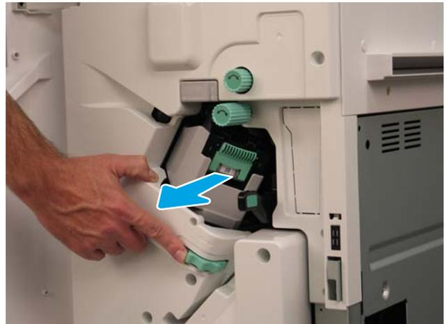
4. Lift two tabs on the staple cartridge, and then lift up to remove the empty staple assembly from the staple cartridge carriage assembly.
