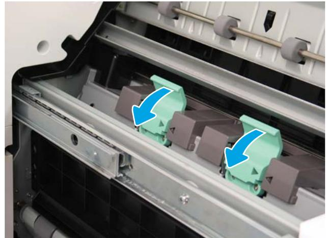
4. Push in the two blue tabs, and then lift up to open the top of the staple cartridge carriage.
