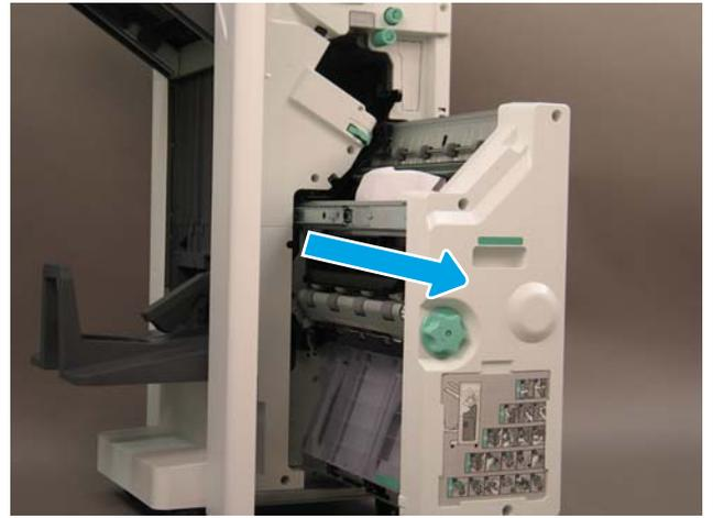
3. Pull the colored tabs away from the assembly, and then pull them up to remove the two staple cartridges.
