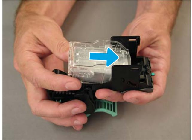
7. Reinstall the two staple cartridge carriages into the booklet maker by pressing the colored handles until they snap into place.
