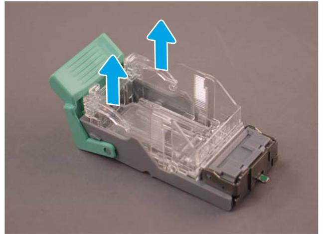
5. Insert the new staple cartridge into the staple cartridge carriage.
