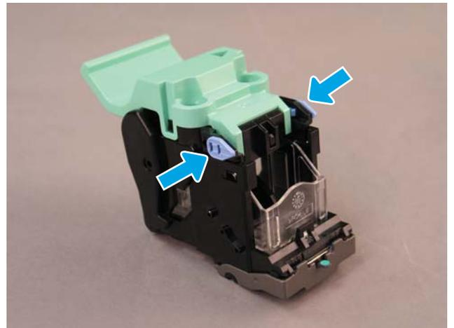
5. Lift two tabs on each staple cartridge, and then lift up to remove the empty staple cartridges from the staple cartridge carriages.
