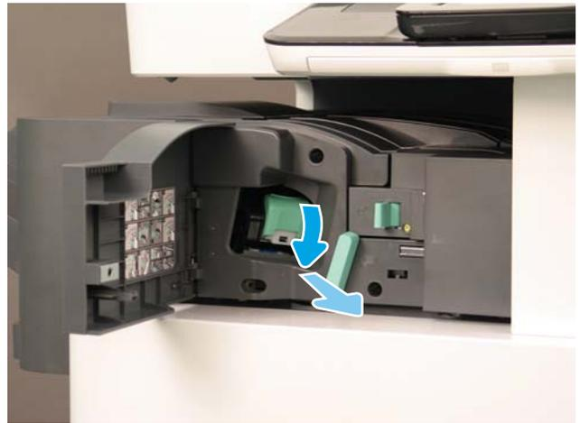
3. Lift two tabs on the staple cartridge, and then lift up to remove the empty staple cartridge from the staple cartridge carriage assembly.
