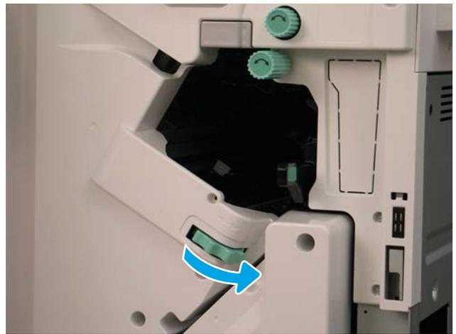
3. Hold the knob to immobilize the staple cartridge assembly, grasp the colored tab on the staple cartridge carriage, and then pull the staple cartridge carriage straight out.
