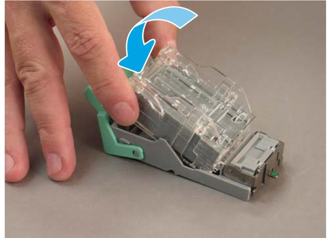
6. Hold the knob to immobilize the staple cartridge assembly, insert the new staple cartridge into the assembly, and then press the colored handle inward until it snaps into place.
