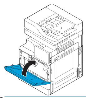
NOTE: If the front door is not closed completely, the printer will not operate.
