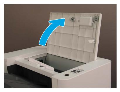
2. Lift the TF feeder, and then turn the knob while the TF feeder is lifted.
