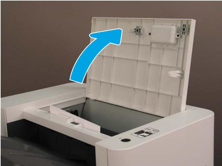
2. Lift the TF feeder, and then turn the knob while the TF feeder is lifted.
