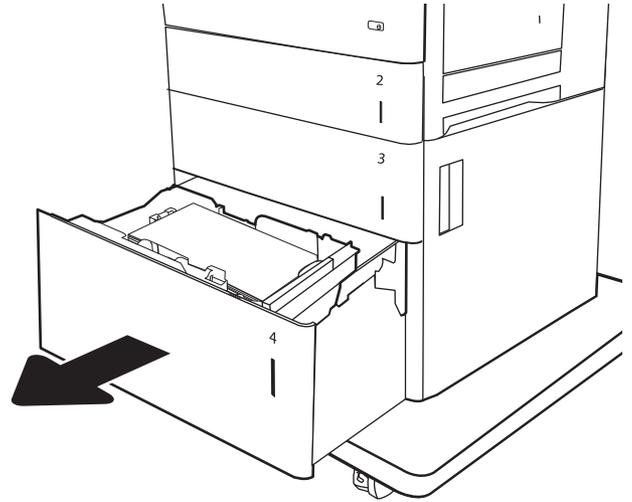
2. Remove any jammed or damaged sheets of paper. Verify that the tray is not overfilled and that the paper guides are adjusted correctly.
