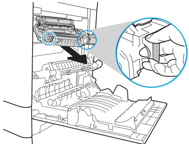
6. Open the jam-access door on the fuser. If paper is jammed inside the fuser, gently pull it straight up to remove it. If the paper tears, remove all paper fragments.
