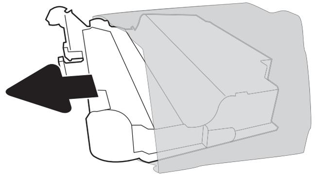
5. Install the new unit into the printer. Make sure the toner-collection unit is firmly in place.
