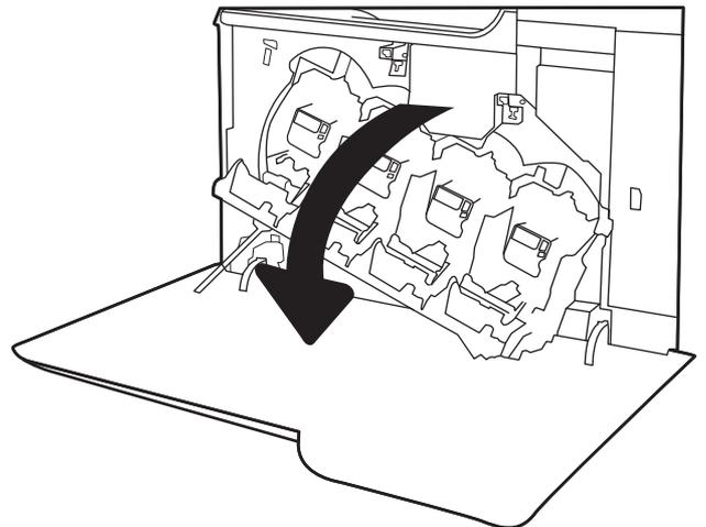
2. Grasp the handle of the used toner cartridge and pull out to remove it.
