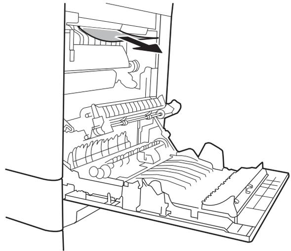
12. Paper could be jammed inside the fuser where it would not be visible. Grasp the fuser handles, lift up slightly, and then pull straight out to remove the fuser.
