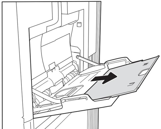
3. Use the blue adjustment latch to spread the paper guides to the correct size, and then load paper in the tray. For information about how to orient the paper, see [Table 2-1 Tray 1 paper orientation on page 22](#).
