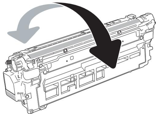
5. Support the toner cartridge underneath with one hand while holding the cartridge handle with the other. Align the toner cartridge with its slot on the shelf, and then insert the toner cartridge into the printer.
