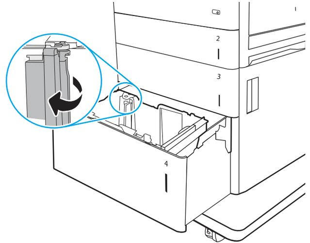
4. Load paper into the tray. Check the paper to verify the guides lightly touch the stack, but do not bend it. For information about how to orient the paper, see [Table 2-3 High-capacity input tray paper orientation on page 32](#).
