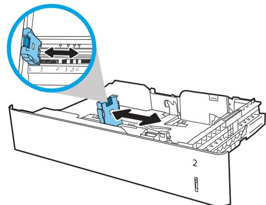
4. Load paper into the tray. Check the paper to verify the guides lightly touch the stack, but do not bend it. For information about how to orient the paper, see [Table 2-2 Tray 2 and the 550-sheet trays paper orientation on page 27](#).
