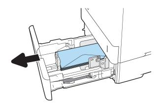
2. Remove any jammed or damaged envelopes from the tray.
