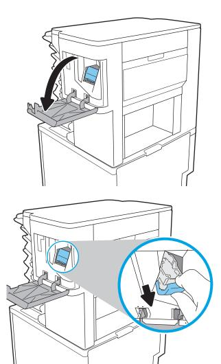
3. Lift up the empty staple cartridge to remove it from the staple carriage.
