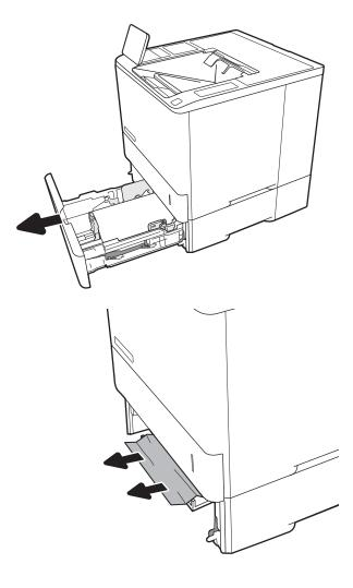
2. Remove any jammed or damaged sheets of paper.
