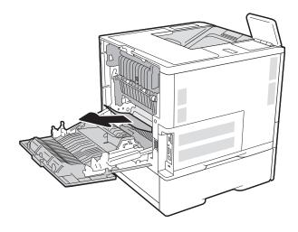
3. Remove the fuser by grasping the two side latches and pulling the fuser straight out of the printer.
