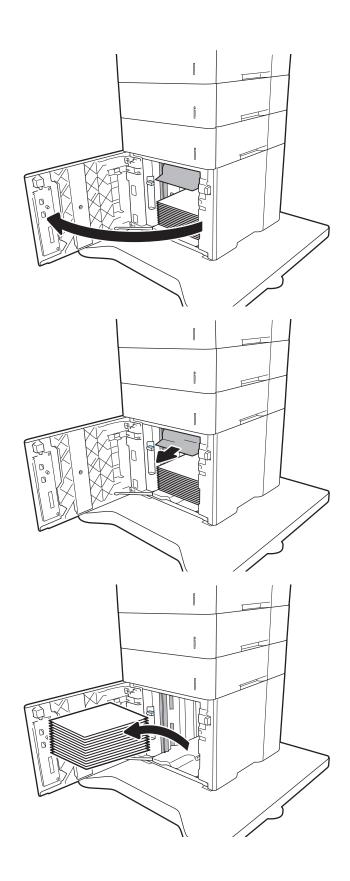
4. If jammed paper is in the feed area, pull it down to remove it.
