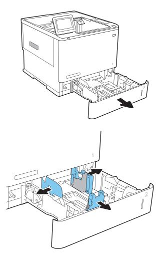
3. Load paper into the tray. Check the paper to verify that the guides touch the stack, but do not bend it. For information about how to orient the paper, see Table 2-2 Tray 2 and the 550-sheet trays paper orientation on page 25.
