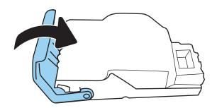
6. Insert the staple cartridge into the stapler and push the colored handle until it snaps into place.
