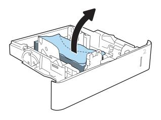
3. Remove any envelopes from the feed rollers inside the printer.
