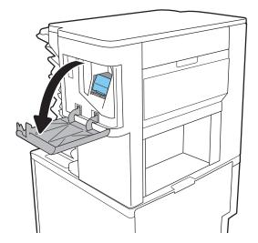
2. Pull the colored handle on the staple cartridge, and then pull the staple cartridge straight out.
