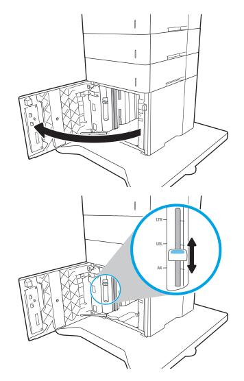
3. Load paper into the tray. Check the paper to verify the guides lightly touch the stack, but do not bend it.
