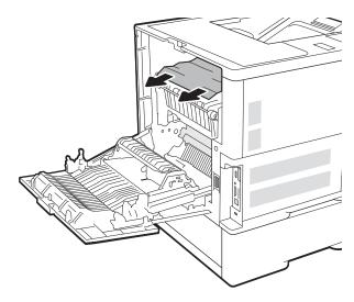
7. Remove any jammed paper from the fuser opening.
