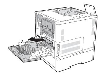
6. Remove the fuser by grasping the two side latches and pulling the fuser straight out of the printer.
