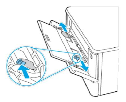
3. Ensure the tray is not overfilled. Paper should be below the 3 triangles in the following image.
