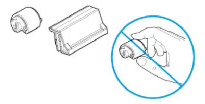
f. Position the pickup roller with the pins in the provided slots on the holder, and then rotate the top of the roller up and toward the printer.
