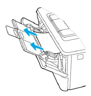
2. Adjust the paper guides to the correct paper size, then .reload paper into the tray.
