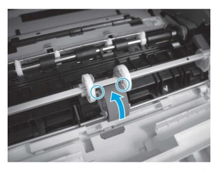
g. Continue to rotate the top of the roller toward the printer (callout 1), until two tabs (callout 2) snap into place.
