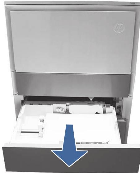
6. Remove the paper from the tray and discard any bent, curled, or damaged sheets.
