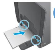
Extend Paper Guides Fully & Load Paper; Adjust Paper Guides to Fit Paper.
