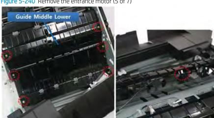
Figure 5-240 Remove the entrance motor (5 of 7)
