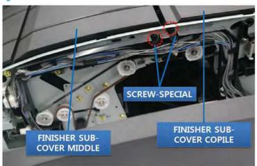
Figure 5-237 Remove the entrance motor (2 of 7)
