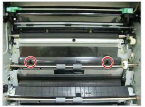
2. Disconnect the connector, remove one screw, and then remove the feed sensor cover.
