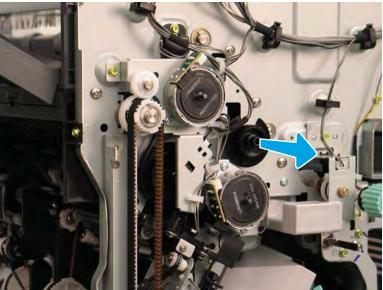
3. If you are replacing the sensor (callout 1), remove it from the motor housing.
