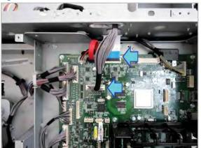
20. Remove three screws. Lift the scanner straight up and off of the printer to remove it.
