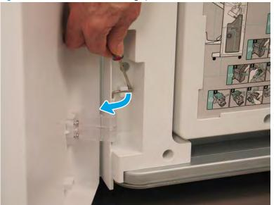
Figure 4-177 Release the lower hinge pin
