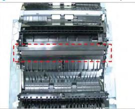
Figure 2-204 Remove transfer roller assembly
