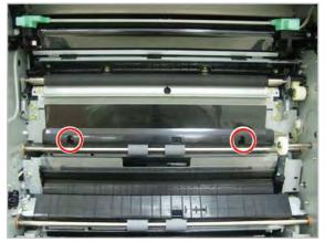
2. Remove the black plastic bushing retainer at the rear of the REGI unit, disconnect one connector, and then remove two screws at the front and rear of the REGI unit.
