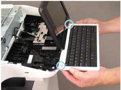
Figure 2–128 Remove the control-panel keyboard
