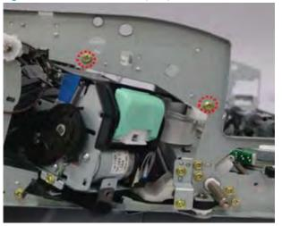
Figure 5-117 Remove the stapler position sensor (1 of 7)
