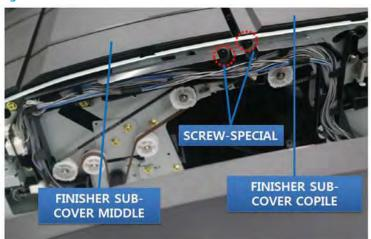
Figure 5-289 Remove the entrance motor (2 of 7)
