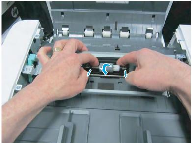
Figure 2-360 Remove the separation roller assembly
