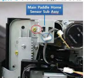
Figure 5-42 Remove the front jogger motor (8 of 22)
