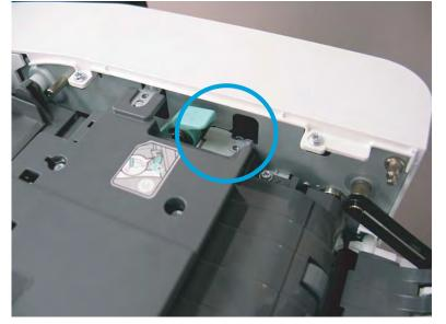
6. To remove the pick/feed roller assembly lift up on the front side (callout 1) and, then slide towards the front (callout 2) to release the pick/feed roller assy.
