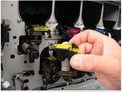
**IMPORTANT:** The toner supply shutters must be in the open (up) position whenever performing service in this area of the printer.
