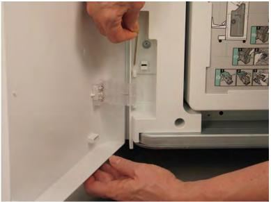
Figure 4-308 Remove the lower hinge pin
