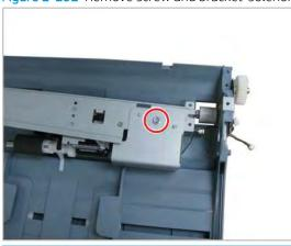
Figure 2-292 Remove screw and bracket-solenoid
