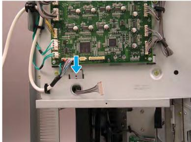
4. Remove one star-washer screw (callout 1), and then release the alignment pin (callout 2) on the right side of the booklet finisher.
