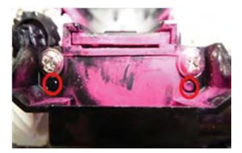
• **Cause**: FRAME MAIN-DUCT Toner assembly does not reach the designated position.
