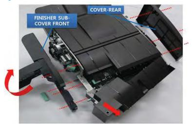
2. Remove two shoulder screws at the rear of the printer, and then remove the finisher sub-cover middle and finisher sub-cover compile by lifting off the hinge pins at the front.
