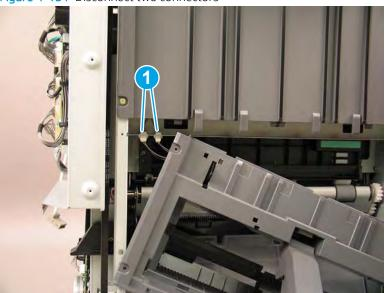
Figure 4-131 Disconnect two connectors
