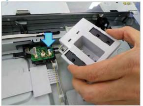
Remove two screws. Release the APS sensor. 4.
