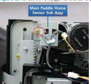
Figure 5-85 Remove the front jogger home sensor (6 of 15)
