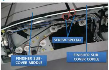
Figure 5-154 Remove the entrance motor (2 of 7)
