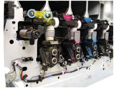
Figure 2-167 Remove the toner duct cover
