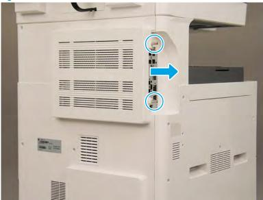
Figure 2-211 Remove the formatter cover
