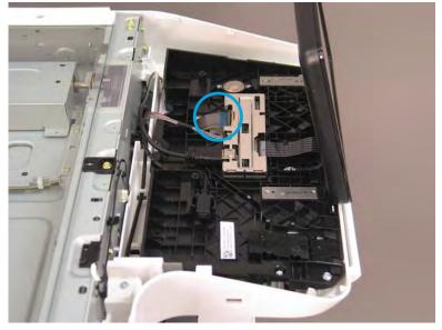
2. Slide the keyboard out, and then depress two latches to remove the keyboard.
