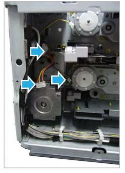
2. Remove three screws, and then remove the feed drive unit.
