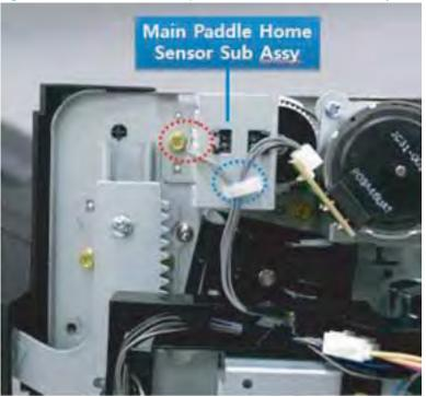
Figure 5-246 Remove the main paddle home sensor sub assembly
