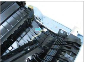
3. Separate the right-door exit after removing three plastic, self-tapping screws.
