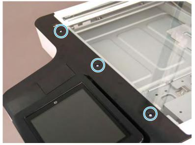
Figure 2-126 Remove the document feeder bezel
