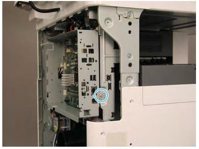
Figure 2-155 Remove the formatter cage side screw
