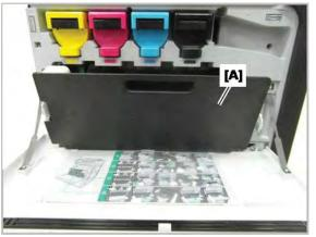
2. Remove the laser scanner assembly window cleaning tool located on the front cover.
