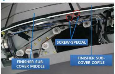
Figure 5-132 Remove the entrance motor (2 of 7)
