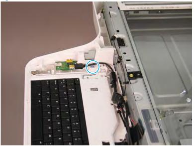
Figure 2-39 Remove USB interconnect cable
