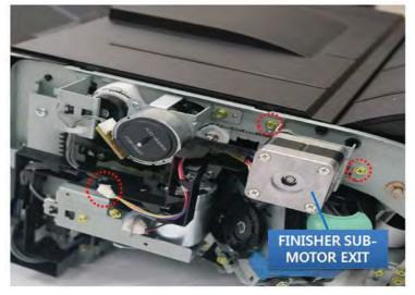
3. Remove the exit motor from the BKT motor feed exit.
