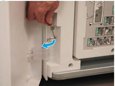
Figure 4-194 Release the lower hinge pin
