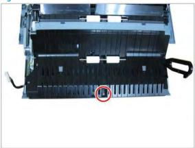
8. Remove two screws from the other side of the door.
