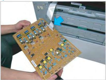
Figure 2-252 Remove the HVPS board
