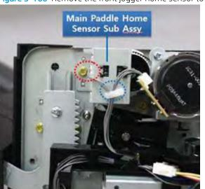
Figure 5-160 Remove the front jogger home sensor (6 of 15)
