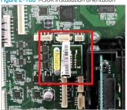
Figure 2-100 MSOK installation orientation
