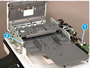
Figure 2-313 Remove the input tray connector, screw, and hinge pin
