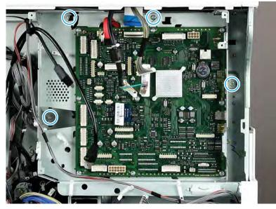
5. Lift the main board cage up slightly to release one bracket, and then pull out to remove.
