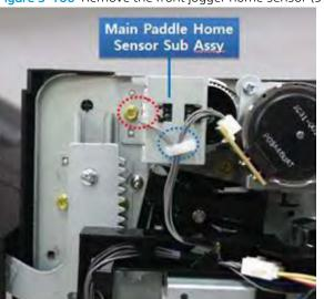
Figure 5-100 Remove the front jogger home sensor (9 of 11)
