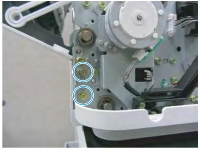
Remove five screws (ADF back; four sheet-metal and one ground). 2.
