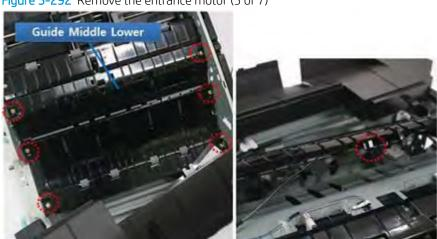
Figure 5-292 Remove the entrance motor (5 of 7)
