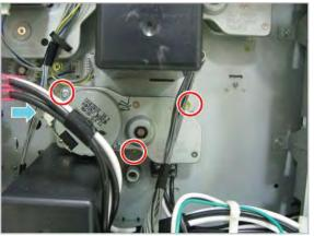
Figure 2-177 Remove screws and pickup drive unit 2
