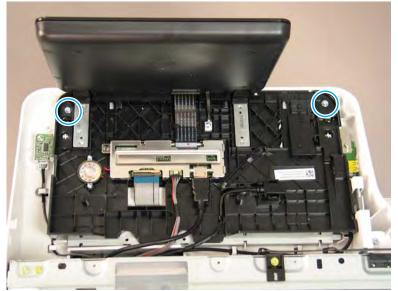
**11.** Disconnect one FFC, one connector, the HIP USB cable, and one HDMI connector.
