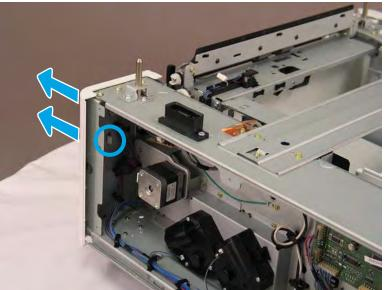
3. Disconnect one connector, and then release the wire harness from the retainer.
