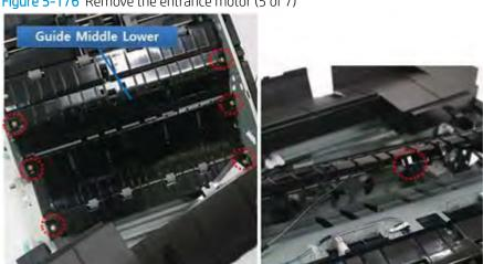
Figure 5-176 Remove the entrance motor (5 of 7)
