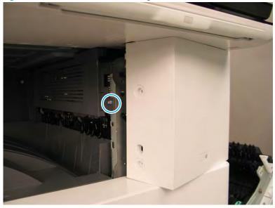
5. Remove four screws and three screw covers. Remove the cover exit rear by pulling from the right and rotating out.
