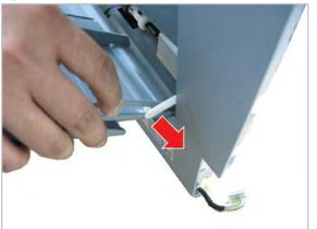
Figure 2-276 Open Tray 1 (MP) and release link
