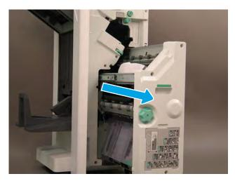
3. Open the vertical tray by pulling outward on the green tab.
