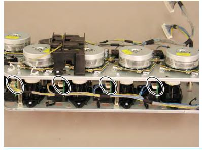
NOTE: To remove the photo interrupters, release the tabs on the back side. Use caution not to damage the plastic hooks.
