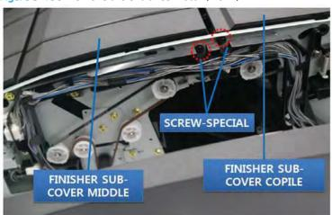
Figure 5-190 Remove the entrance motor (2 of 7)
