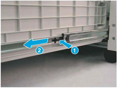
Figure 2-575 Release the tray right-side slide lock
