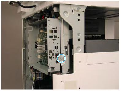
Figure 2-87 Remove the formatter cage side screw
