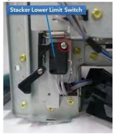
**13.** Open three clamps, unplug the connector, and then remove the sensor.
