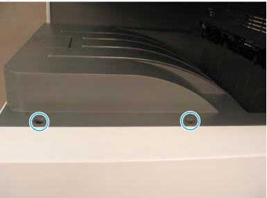
Figure 2-119 Remove screw-caps and screws
