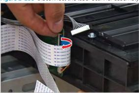
Figure 2-255 Disconnect the laser scanner assembly harness and FFC cable
