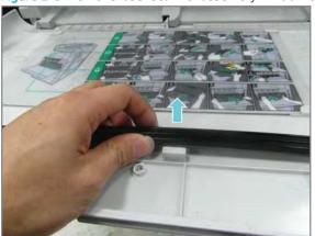
3. Insert the laser scanner assembly window cleaning tool into each color entrance.
