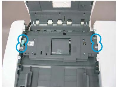
2. Remove two screws on the front cover.
