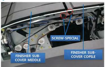
Figure 5-19 Remove the entrance motor (2 of 7)
