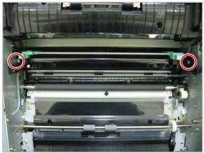
3. Remove the ITB unit until the handles are fully visible. Release the ITB unit smoothly.
