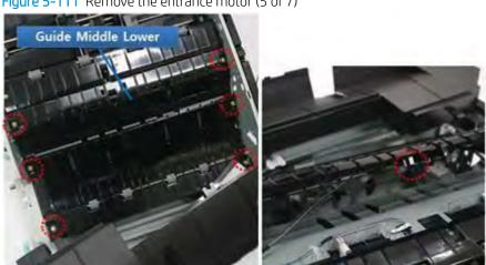
Figure 5-111 Remove the entrance motor (5 of 7)
