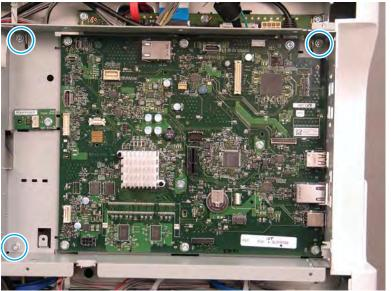
Figure 2-156 Remove three screws to remove the formatter cage
