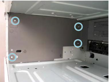
Figure 2-121 Remove screws and cover exit rear
