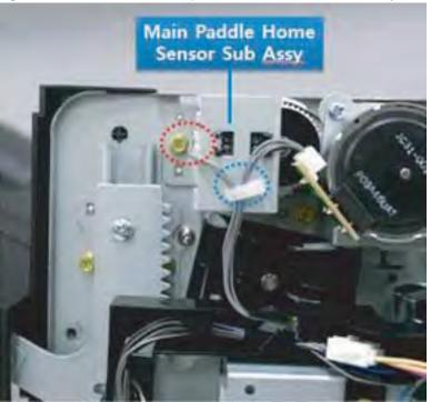
Figure 5-182 Remove the main paddle home sensor sub assembly
