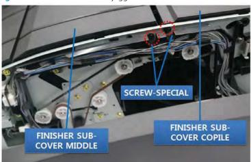
Figure 5-36 Remove the front jogger motor (2 of 22)
