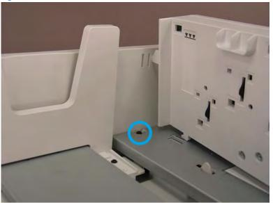
5. Raise the paper shelf, hold the sub-paper side right assembly up and out of the way, and then remove the sheet-metal cover.
