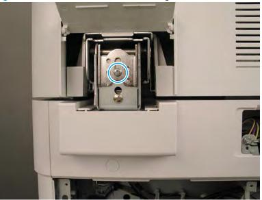
Figure 2-23 Release the document feeder hinge screws
