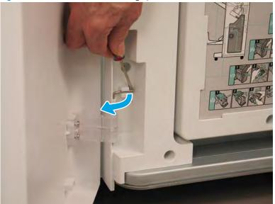
Figure 4-379 Release the lower hinge pin
