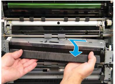
2. Release the small tab and remove the pick/feed/separation roller. Note the location of the clutches and gears.
