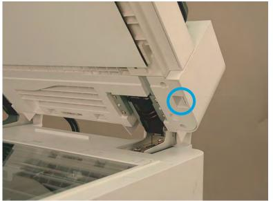
4. Release the three tabs on back cover to remove the back cover.
