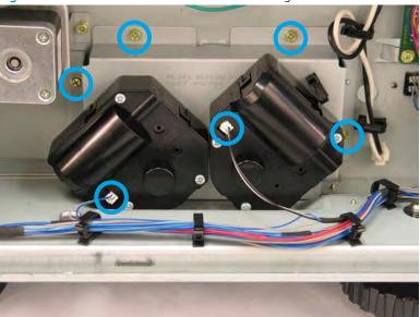
Figure 2-547 Remove the HCI motor - lift drive right and motor - lift drive left
