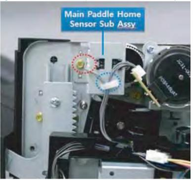
Figure 5-271 Remove the main paddle home sensor sub assembly
