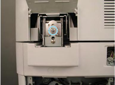
Figure 3-81 Adjust ADF hinge
