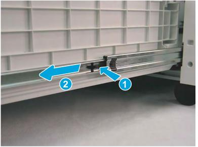
Figure 2-566 Release the tray right-side slide lock
