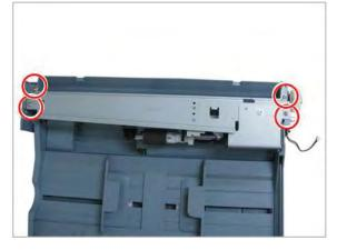
20. Release the cable from the cable retainer, and release the cable from the cable harness. Remove two screws, and then remove the MP solenoid.
