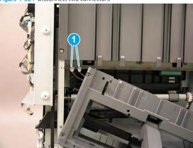
Figure 4-321 Disconnect two connectors
