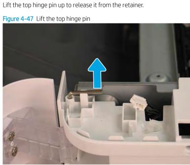
2. Pull the top hinge pin up to remove it.
