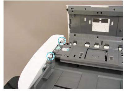
2. Remove three screws from the bottom of the document feeder front cover, and then remove the document feeder front cover.
