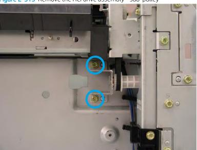
Figure 2-519 Remove the HCI drive assembly - sub-pulley
