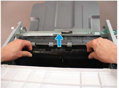
Figure 4-208 Remove the feed assembly
