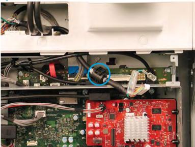
Figure 2-26 Remove the cable choke
