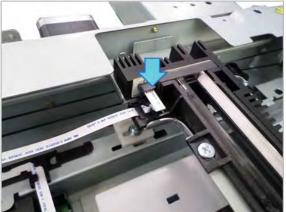
3. Remove four screws. Release the LED lamp module.
