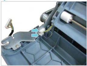
**14**. Remove one screw, and then remove the Tray 1 unit.
