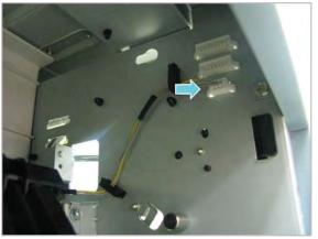
2. Remove three screws, and then remove the exit unit.
