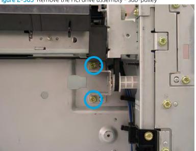
Figure 2-563 Remove the HCI drive assembly - sub-pulley
