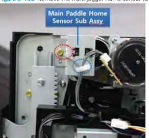
Figure 5-196 Remove the front jogger home sensor (6 of 15)
