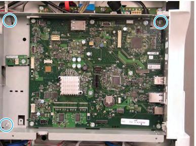
Figure 2-88 Remove three screws to remove the formatter cage
