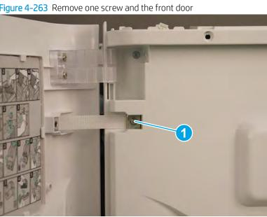
Figure 4-263 Remove one screw and the front door
