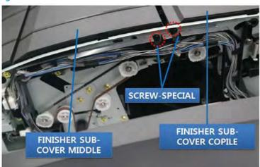
Figure 5-166 Remove the entrance motor (2 of 7)
