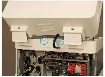
2. Remove the plastic cable choke from the wire harness, and then disconnect the document feeder harness from the main board. Disconnect the insulated ground wire from the chassis.
