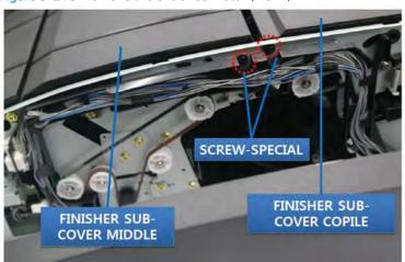
Figure 5-216 Remove the entrance motor (2 of 7)
