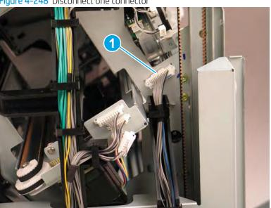
Figure 4-248 Disconnect one connector
