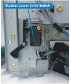
**11.** Open three clamps, disconnect the connector, and then release the switch.
