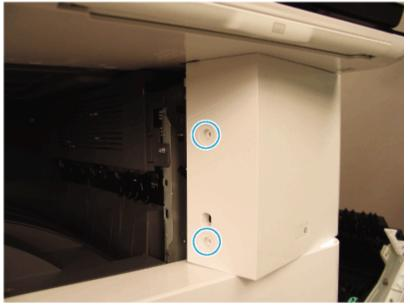
3. Remove two screw-caps and two screws, and then remove the exit tray.
