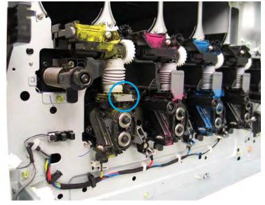
2. Remove the shutter from the top of the developer unit.
