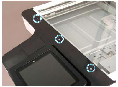
Figure 2-123 Remove the document feeder bezel
