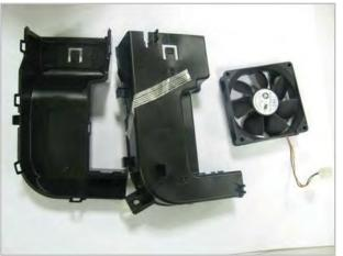
**CAUTION:** When installing the new fan, make sure not to change the fan direction. The label must be visible on the outside of the fan.
