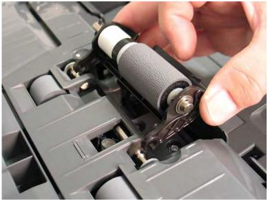
Figure 2-402 Remove the separation roller
