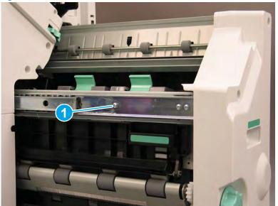
7. Lift the booklet finisher up on the left side while squeezing the right rail away from the finisher slightly to clear the sheet metal. Remove the booklet finisher.
