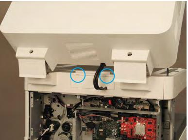
2. Remove the connector and one screw.
