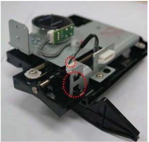
**23.** Remove the tamper front sub assembly.
