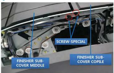
Figure 5-27 Remove the entrance motor (2 of 7)
