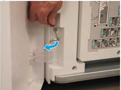
Figure 4-261 Release the lower hinge pin
