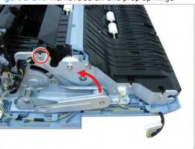
Figure 2-279 Remove screw and prop up hinge
