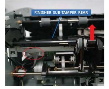
**16.** Remove two screws, unplug the connector, and then remove the rear jogger motor.
