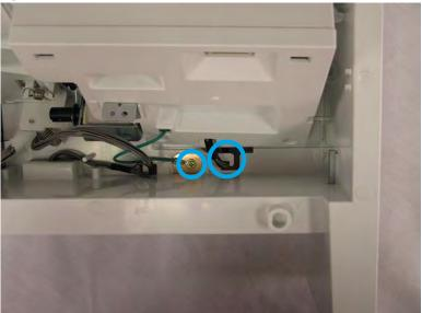
Figure 2-569 Remove one screw and release the wire harness
