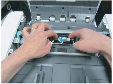
Figure 3-57 Remove the separation roller assembly
