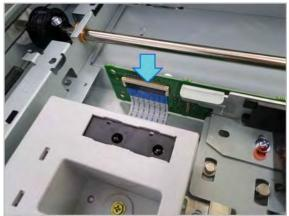
3. Remove two screws and release the scanner imaging unit.
