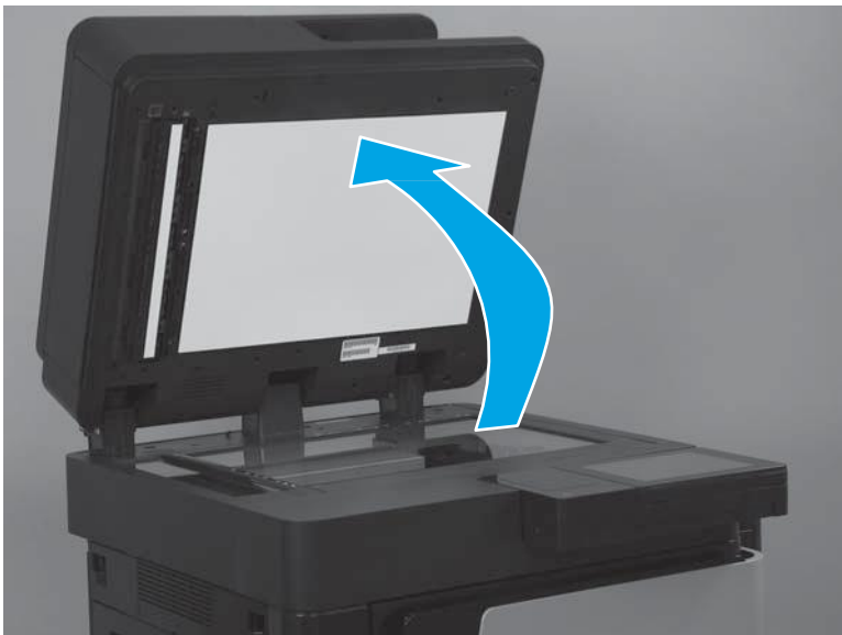
Figure 28. Install a replacement document feeder white backing (M880; 5 of 6)
