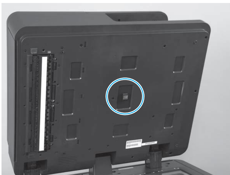
Figure 23. Remove the document feeder white backing (M880; 3 of 3)
