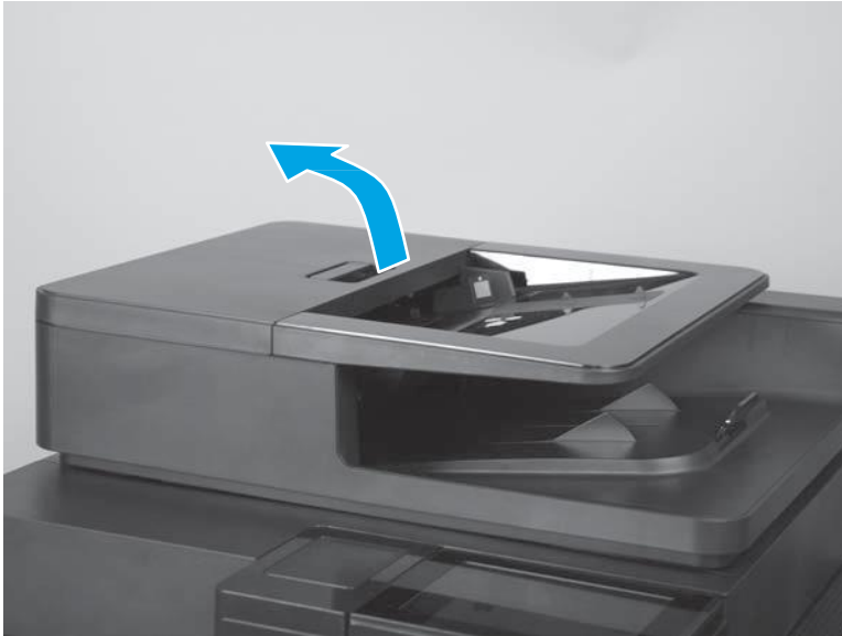
Figure 30. Remove the background selector (M880; 1 of 4)
