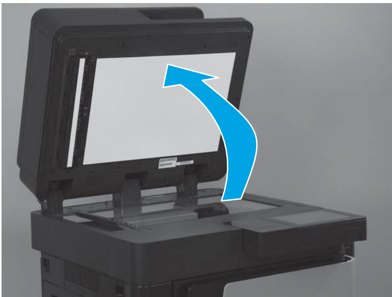
Figure 21. Remove the document feeder white backing (M880; 1 of 3)
