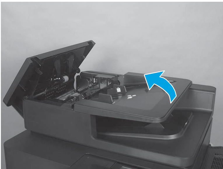
Figure 31. Remove the background selector (M880; 2 of 4)
