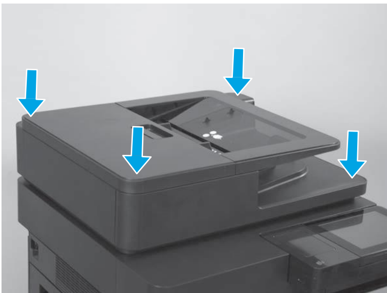
Figure 27. Install a replacement document feeder white backing (M880; 4 of 6)
