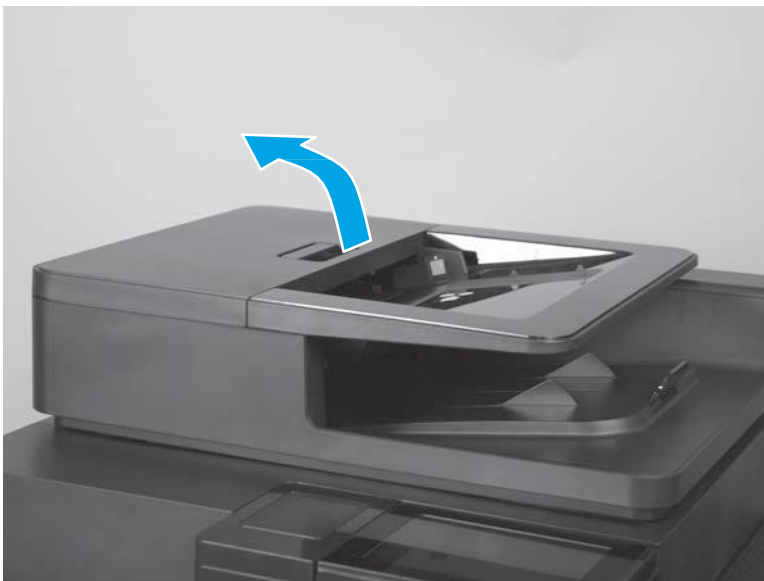
Figure 15. Remove the document feeder mylar strip (M880; 1 of 4)
