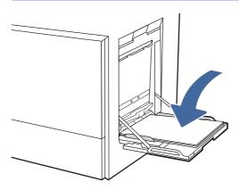
5. Using the adjustment latch, adjust the side guides so that they lightly touch the paper stack, but do not bend it.
