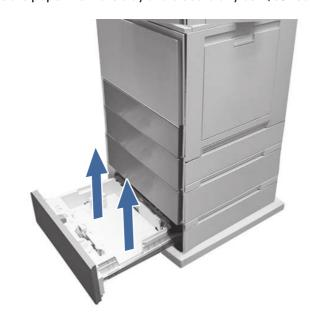
9. Make sure that the tray width and length guides are set to the correct paper size for the paper being installed into the tray and that the tray is not over filled above the fill mark (line below 3 triangles on rear guide).
