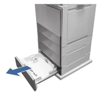
8. Remove the paper from the tray and discard any bent, curled, or damaged sheets.
