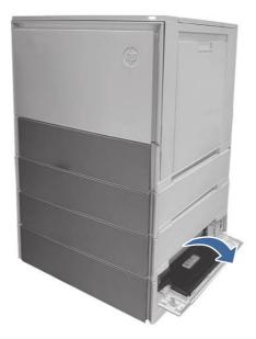
b. Locate and remove the Tray 5 separation roller.
