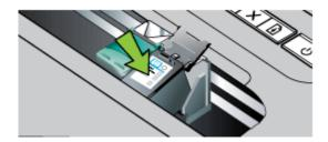
**5.** Close the ink cartridge latch. If the cartridge is inserted correctly, closing the latch gently pushes the cartridge into its cradle compartment. Press the latch to make sure it is seated flat on the cartridge.
