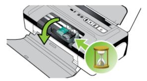
**3.** Lift the ink cartridge latch open and gently remove the ink cartridge from its cradle compartment.
