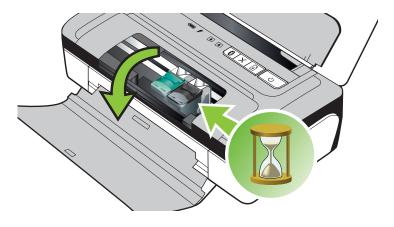
**3.** Wait until the print carriage is idle and silent, and then lift up the ink cartridge latch to release the ink cartridge.
