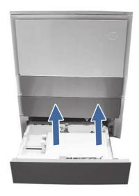
9. Make sure that the tray width and length guides are set to the correct paper size for the paper being installed into the tray and that the tray is not over filled above the fill mark (line below 3 triangles on rear guide).
