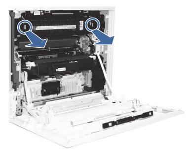
b. Remove any paper jammed in the fuser exit area.
